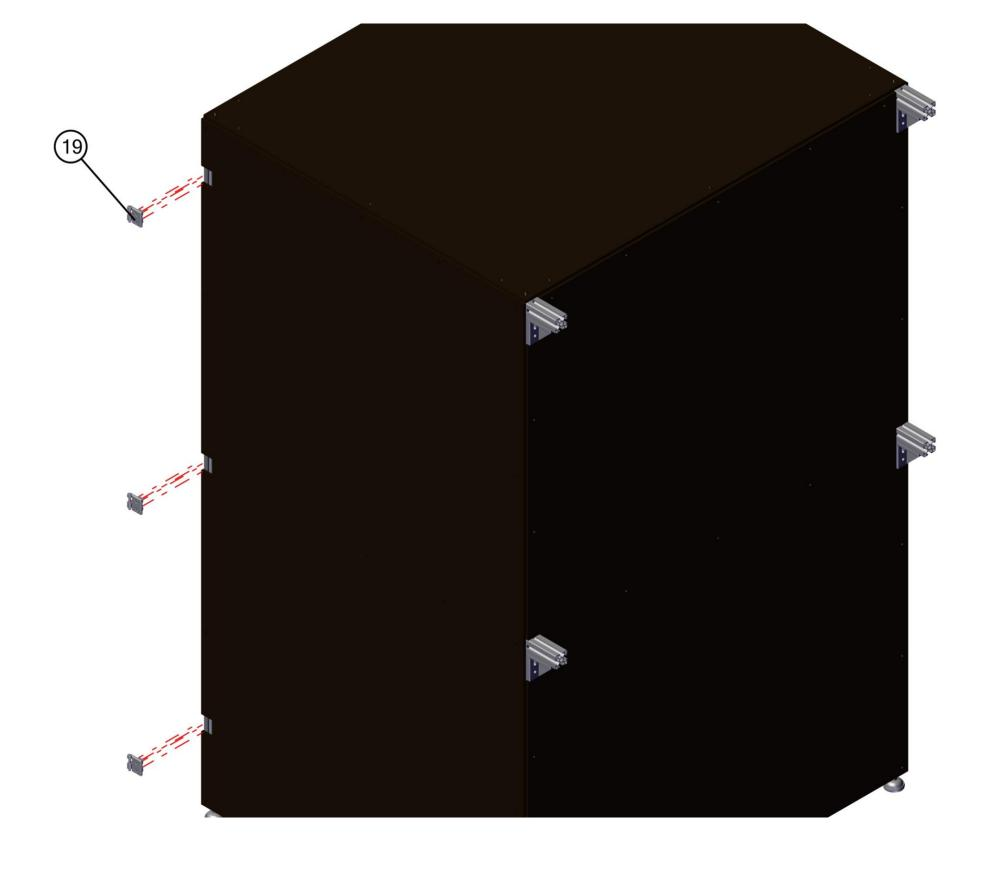
Use the half of the hinges and the supplied screws and nuts.
