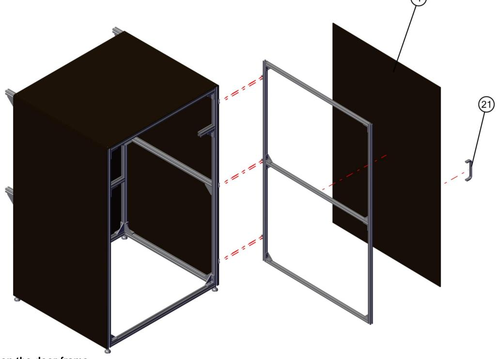
Fix the board 4 and item 21 on the door frame. Then hinge the door.
