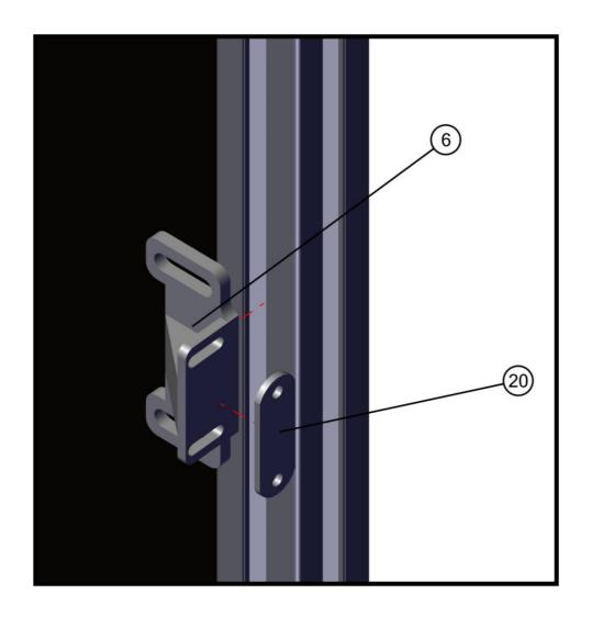
On one side of the door, attach to the profile the Magnet bracket with the magnetic plate supplied with item 20.
