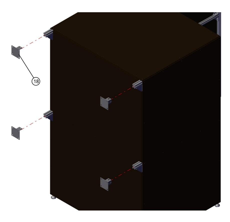
Use the supplied screws and nuts to fixe items 18 the profiles.
