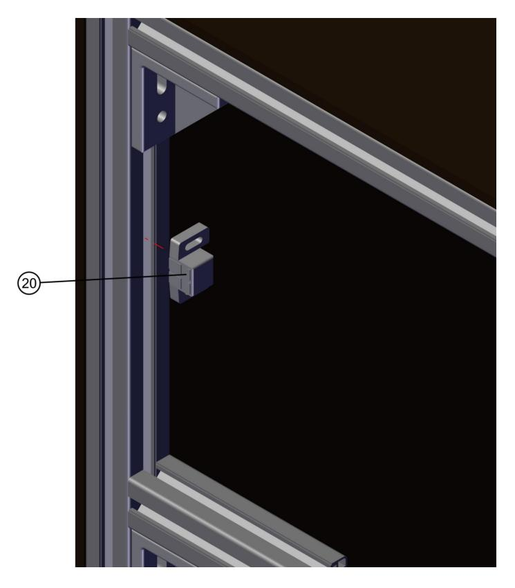
On the other side, fix item 20 with the supplied screw and nuts.
